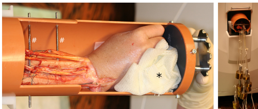
Fig. 1. Left: positioning and fixation of the forearm within the custom made HR-pQCT sample holder, fixed with screws (#). The figure shows the wrist in radial abduction. The white material (*) is plastic cast roll which was used to impose the wrist position and stabilize it during scanning. Right: sample holder placed into the HR-pQCT scanner with weights simulating muscle forces.
