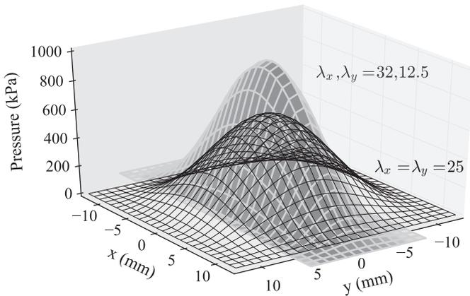
**Fig. 1.** Pressure model Eq. (1). Depicted are a symmetrical pulse with a wavelength of  $\lambda = 25$  mm, an asymmetrical pulse with  $\lambda_x = 32$  mm and  $\lambda_y = 12.5$  mm. Maximum pressures are 640 and 1000 kPa, respectively, and both pulses describe a total force of 100 N.
