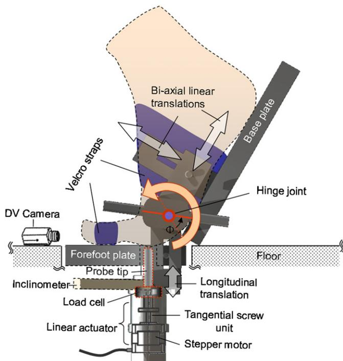
**Fig. 1.** Schematic diagram of the sub-Metatarsal Pad Elasticity Acquisition Instrument (MPEAI), showing details of probe tip, accommodation of sub-MTH pad, and inside components of actuator to drive probe tip.
