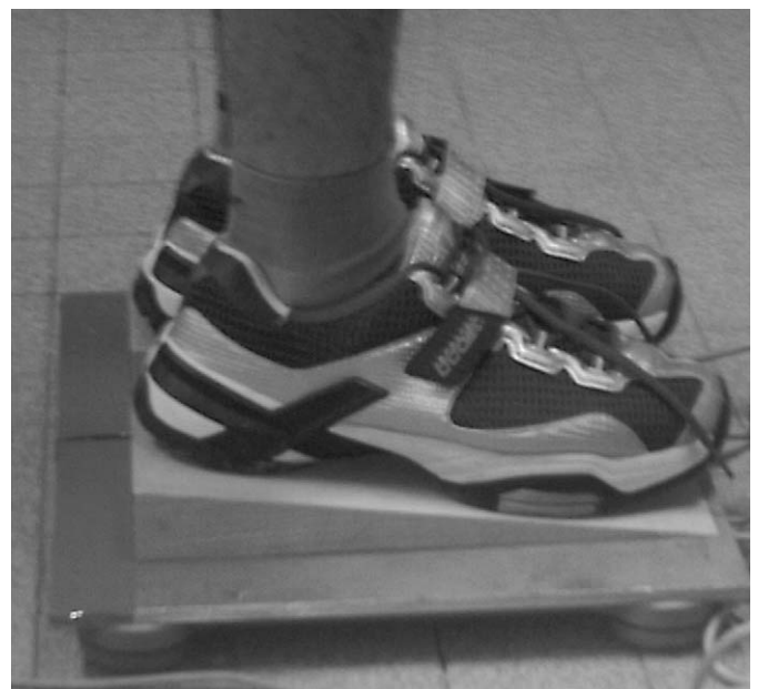
Fig. 1. Photograph showing the force platform device, the wedges, and the shoes used in this study. Note that the displayed wedges position causes a plantarflexion instead of a dorsiflexion.
