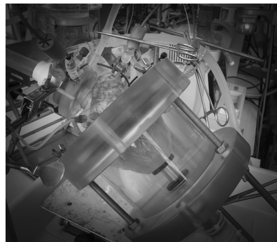
Fig. 2. Picture of the platform showing the heart housed in the fluid-filled chamber.
