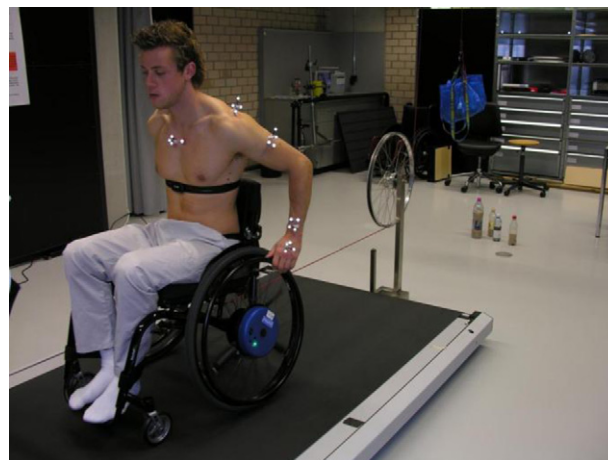
Fig. 1. Overview of the test setup where the subject is propelling against extra resistance generated by a pulley system.
