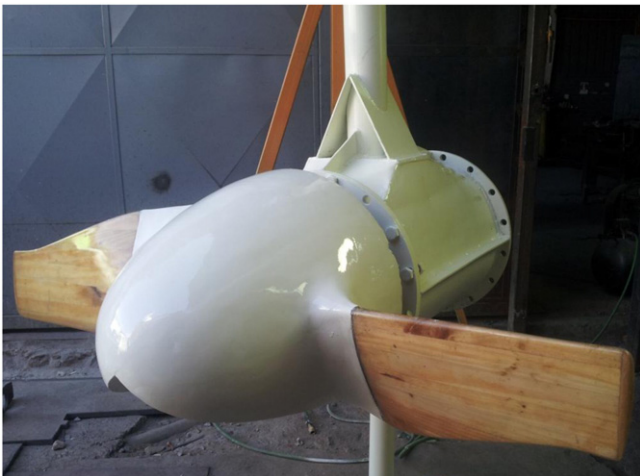
Fig. 1. 5 kW Horizontal axis hydrokinetic turbine designed with Turbem.
