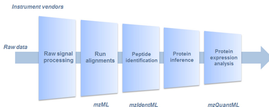
Fig. 1. Prototypical workflow for a label free quantitative analysis, showing which stages are covered by different PSI formats.
