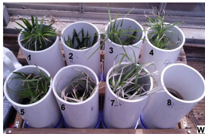
Fig. 1. Ammonia stress on C. alternifolius demonstrated by eight microcosms (W1–W8) after one week of batch operation with dairy wastewater at different initial ammonia concentrations, i.e., 33, 51, 94, 147, 193, 293, 400, and 194 mg N/L in W1–W8, respectively. W1–W7 with C. alternifolius and W8 without plants.
