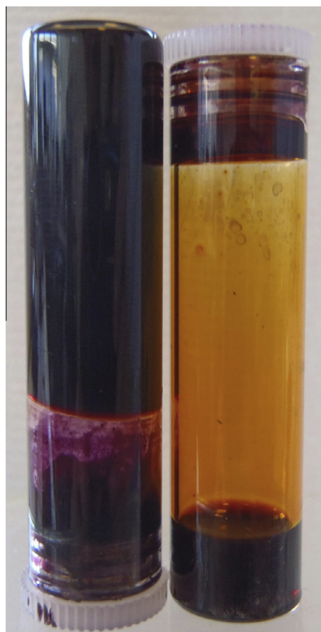
Fig. 2. Photos of the P3HT:PCBM blend: (left) A gel formed from the modified blend; (right) the liquid blend of the unmodified P3HT:PCBM in chlorobenzene.
