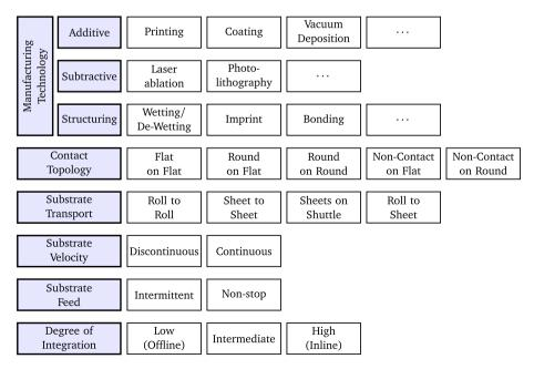
Fig. 1. Classification of substrate-based manufacturing processes.
