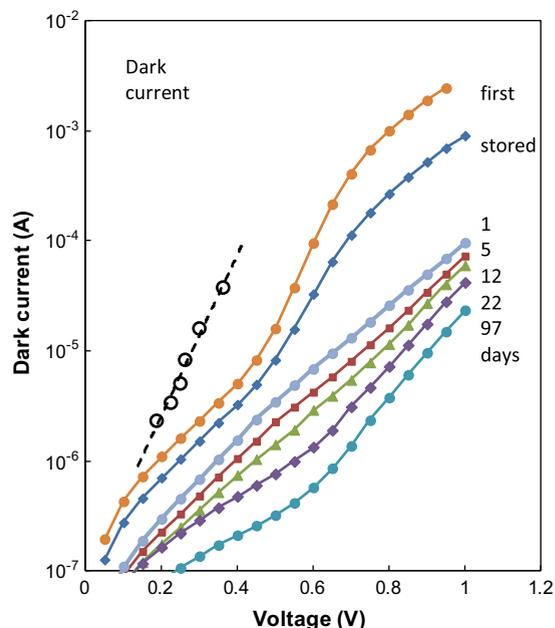
Fig. 1. Plot of the voltage dependence of the forward bias dark current for the unencapsulated organic solar cell after various stages of exposure to the ambient, extending for 97 days. Open circles and dashed line shows the voltage difference between the first and 5 day data.
