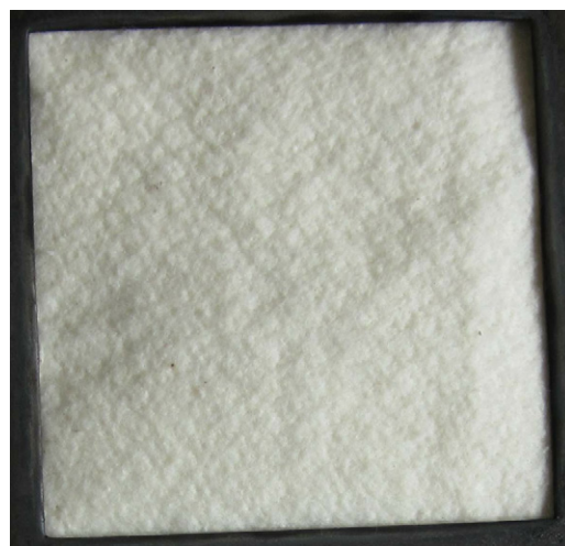
Fig. 1. UCF sample in sample holder before testing on cone calorimeter.
