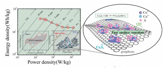
$\label{eq:coss-linked} Cross-linked \quad and \quad robust \quad Co_9S_8/graphene \quad (CoSG) \quad hybrid \quad electrode \quad with \quad remarkable \\ pseudocapacitive features was designed for high-rate hybrid supercapacitors (HSCs).$
