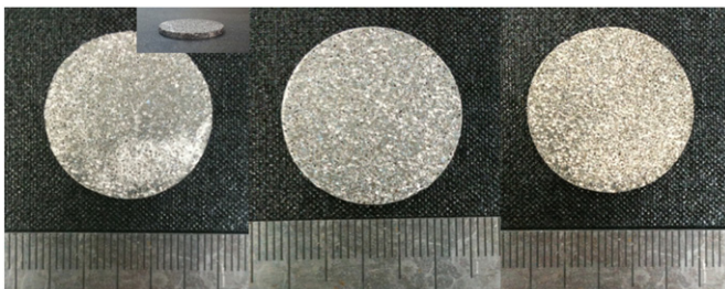
Fig. 2. Typical optical images of the porous Ti scaffolds produced with various initial Mg contents (50, 60 and 70 vol.%, left to right).
