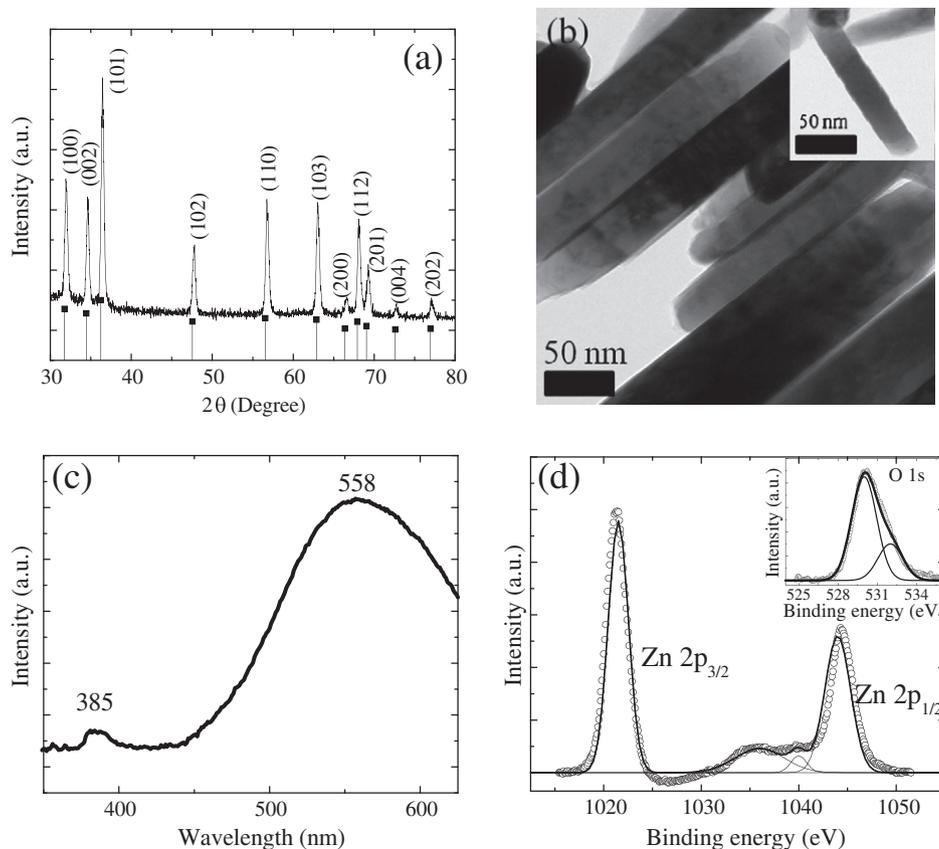
Fig. 1. (a) XRD, (b) TEM [inset shows single rod], (c), PL of the ZnO, and (d) XPS of zinc [inset shows XPS of oxygen].
