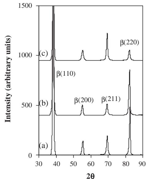
Fig. 1. X-ray diffraction patterns of solution treated Ti–35Nb–7Zr–5Ta containing (a) 0.06, (b) 0.46 and (c) 0.68 wt.% O.
