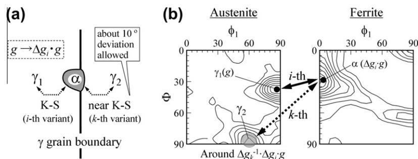
Fig. 1. Schematic representations of (a) the double K–S relation and (b) its influence on variant selection.
