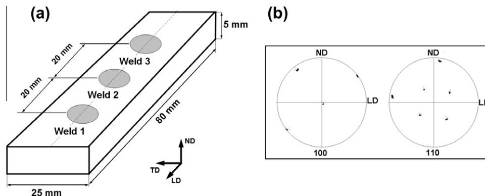
Fig. 1. Schematic of single-crystal sample with employed reference frame (a) and 100 and 110 pole figures showing crystallographic orientation of the single crystal (b). Note: LD, TD and ND are longitudinal, transverse and normal directions, respectively. See text for details.
