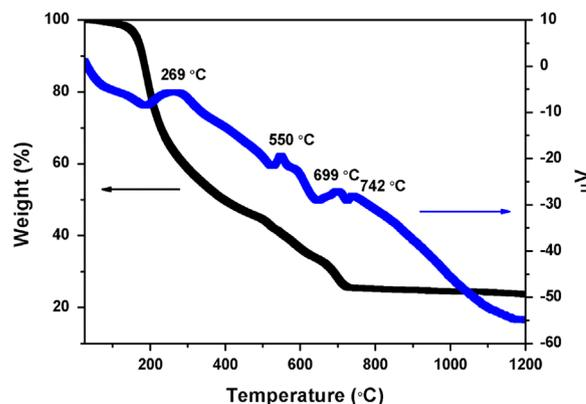
Fig. 1. TG/DTA curves of  $\text{CaGd}_2(\text{MoO}_4)_4\text{:Eu}^{3+}$  powder precursor.
