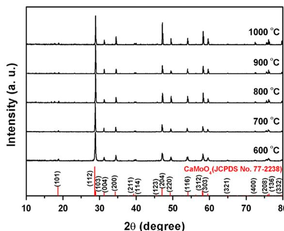
Fig. 2. X-ray diffraction patterns of  $\text{CaGd}_2(\text{MoO}_4)_4\text{:3Eu}^{3+}$  phosphors as a function of annealing temperature.
