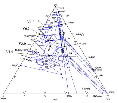
Fig. 1. Phase equilibrium diagram for the  $Na_2O-Al_2O_3$  system<sup>25</sup> showing the primary crystalline phase fields, isotherms and binary and ternary invariant point temperatures.
