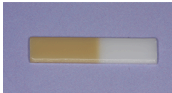
Fig. 1. A photo showing a 20 mm long bi-colored zirconia test bar prepared for four-point bending test.
