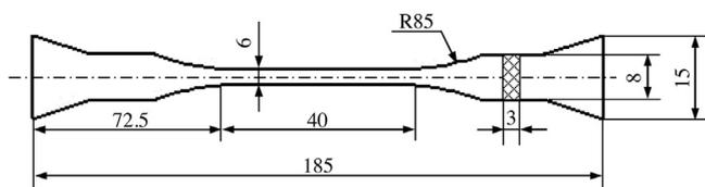
Fig. 1. Shape and sizes of the C/SiC-BC<sub>x</sub> composites specimen.
