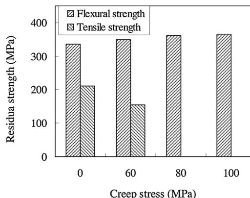
Fig. 3. The normalized residual strength of 2D C/SiC-BC<sub>x</sub> composites after creeping under different tensile stress at 900 °C.
