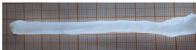
Fig. 2. The picture of the longest mullite crystal grown at a rate of 10 mm/h.
