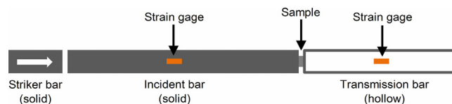
Fig. 2. Schematic of a modified split Hopkinson pressure bar (SHPB) set up for testing foams.
