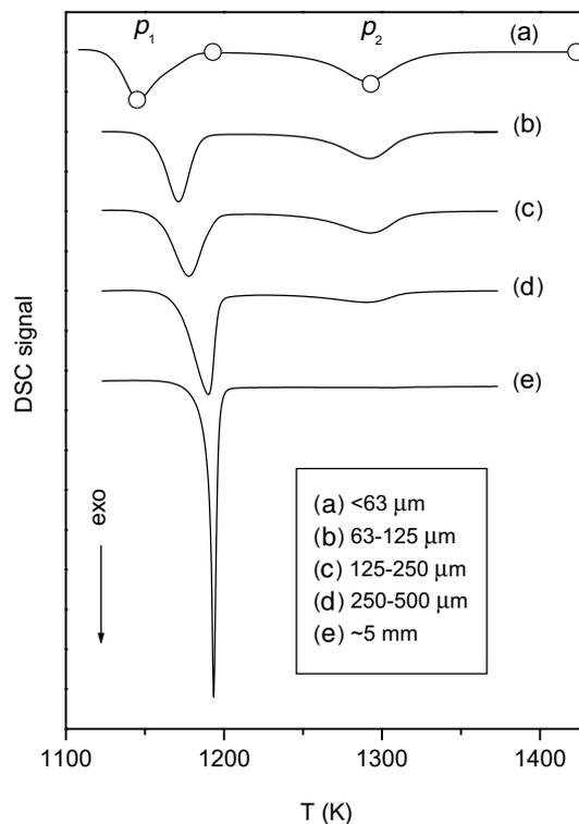
Fig. 1. DSC scans for non-isothermal crystallization of glasses as a function of particle size, (heating rate 10 K min<sup>-1</sup>). (a) glass particles <63 μm; (b) glass particles 63–125 μm; (c) glass particles 125–250 μm; (d) glass particles 250–500 μm, (e) glass particles ~5 mm. Scans are shifted for visualization purposes. Circles on DSC scan (a) assign the quench temperatures for subsequent XRD analyses.
