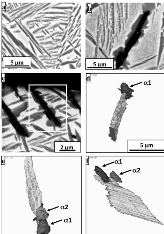
**Figure 1.** Microstructures of (a) base Ti5553 alloy, (b) Ti5553-0.5B alloy, (c) TiB selected for serial sectioning and (d–f) TiB and associated  $\alpha$  in a 3-D view.
