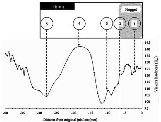
Fig. 1. Schematic of weld transverse plane (retreating side) showing locations used for TEM examination together with their associated hardness values.
