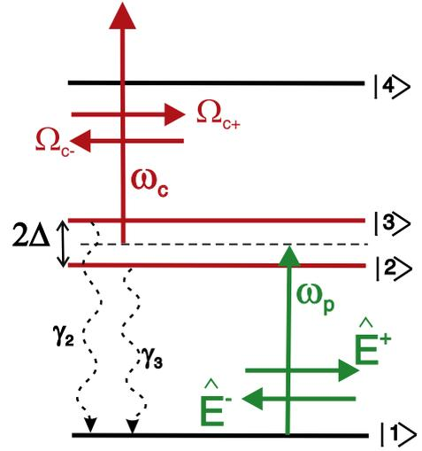
Fig. 1. Four-level scheme in the  $V-\Lambda$  configuration. Forward and backward propagating control fields with Rabi frequencies fields  $\Omega_{c\pm}$  and a weak signal field  $\hat{E}_{\pm}$ .
