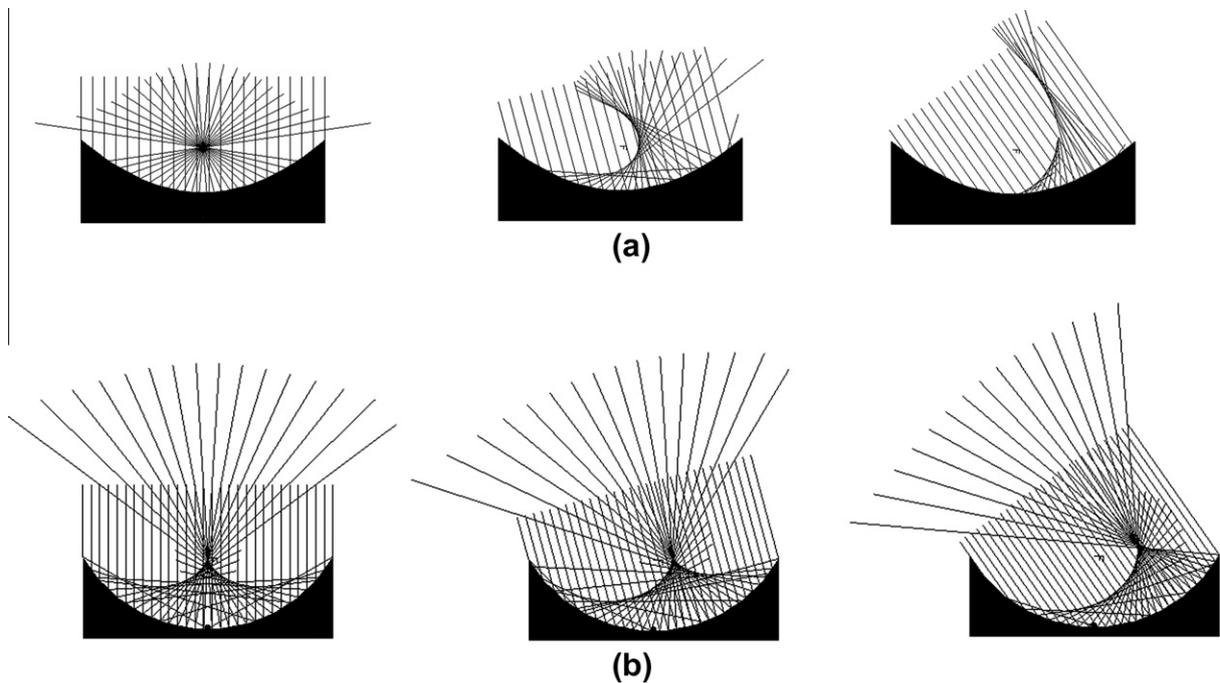
Fig. 1. Incident sunlight (shown as parallel lines) on (a) a parabolic mirror, and (b) a circular mirror, at the angles indicated. The parabolic mirror focuses only the axially incident radiation to a point. Radiation reflected from the circular mirror is not focused to a point. However, at all incident angles, the area of focused radiation has the same mathematical form albeit in a different place.
