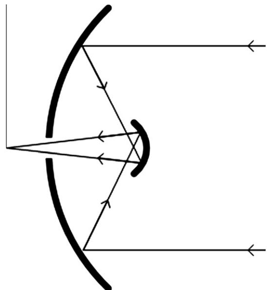
Fig. 2. Diagram of a Gregorian telescope.
