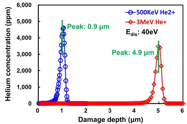
Fig. 1. Irradiation damage profile of 3 MeV and 500 KeV helium ions as a function of the depth, calculated using SRIM software.
