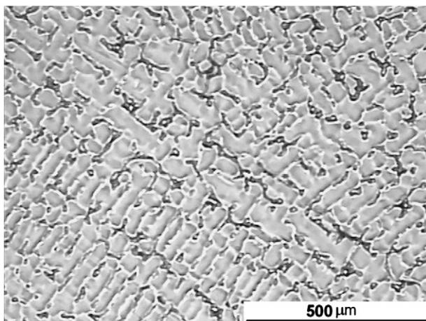
**Fig. 1 – Optical micrograph of the as-cast microstructure of C1 at the upper section.**
