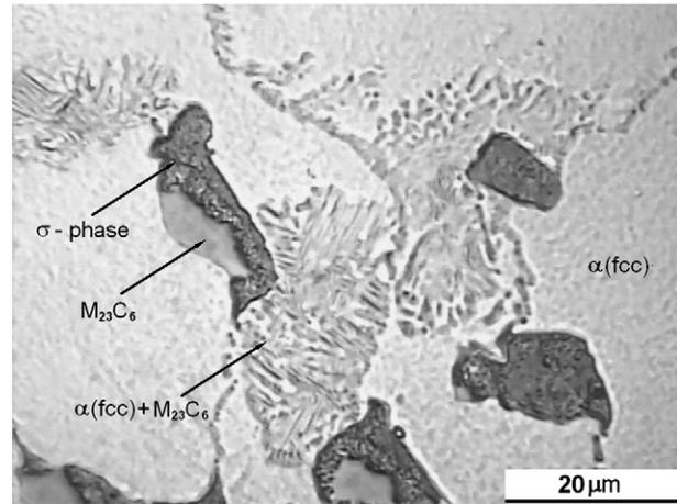
**Fig. 2 – OM for C1, color detected phases are shown.**
