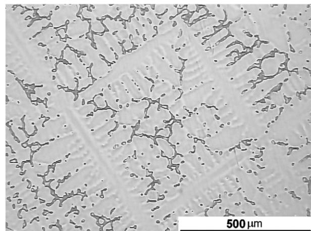
**Fig. 3 – Optical micrograph of the as-cast microstructure of C1 at the bottom section.**
