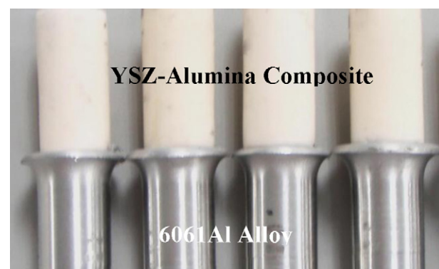
Fig. 2. Overview of friction welded YSZ–alumina composite with 6061 Al alloy joints.
