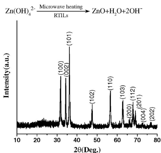
Fig. 1. A typical XRD pattern of as-prepared sample.
