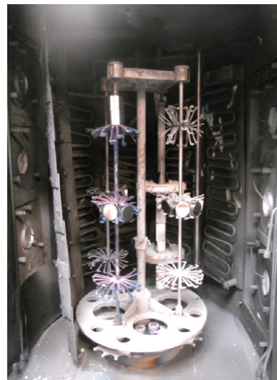
Fig. 1. Schematic and real image of the coating deposition system used in this investigation.
