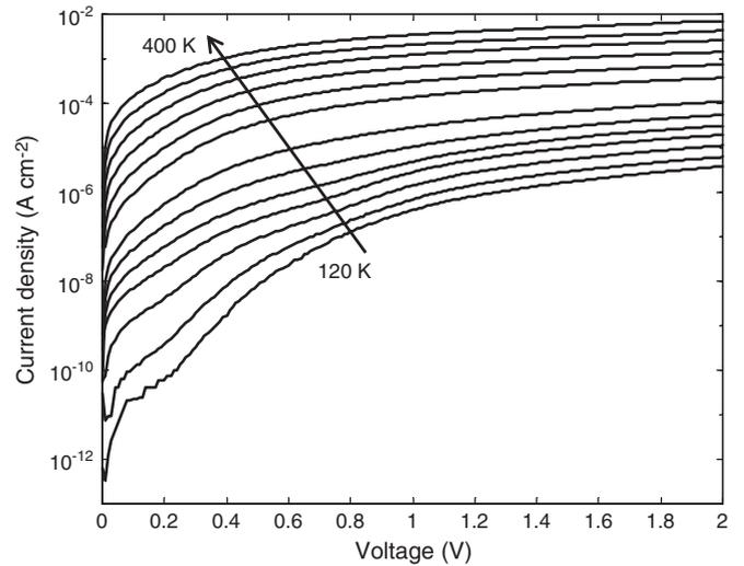
Fig. 1. Experimental forward bias current–voltage characteristics of the CVD diamond/silicon junction at various temperatures.
