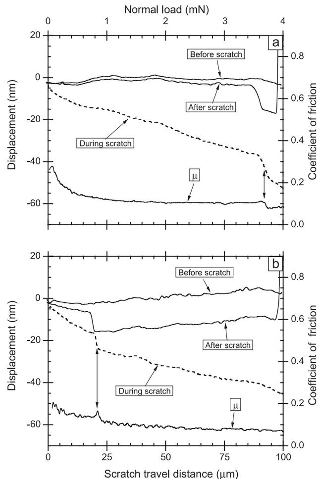
Fig. 1. Ramped load (4 mN) nanoscratch surface displacement and friction coefficient profiles for Au/D/SiO<sub>x</sub>/Si (a) and Au/SiO<sub>x</sub>/Si (b).
