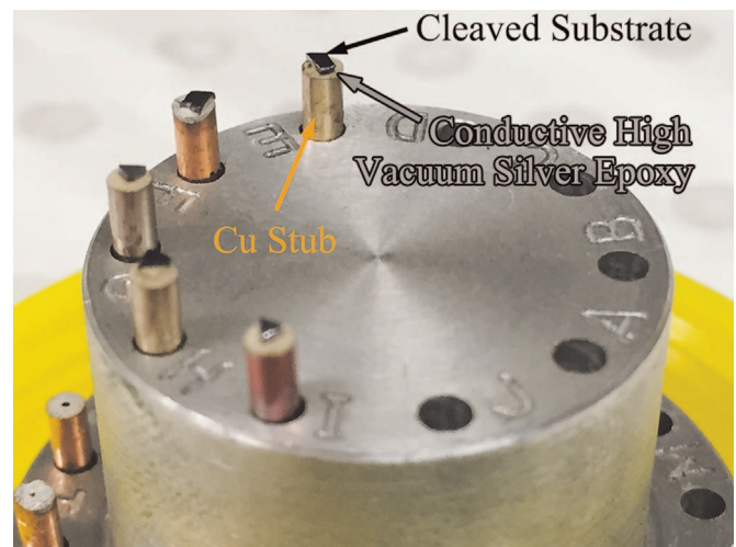
Fig. 2. Cleaved substrates are attached on Copper stubs with conductive high vacuum silver epoxy.
