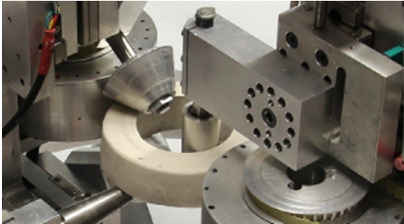
Fig. 3. Model ring rolling machine at University of Cambridge.
