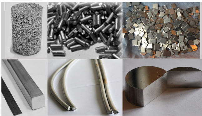
Fig. 1. Scrap input (up) and fully dense profiles and near-net shape semi-finished products (down) obtained from the ECAP hot extrusion, screw extrusion and SPS processes respectively.
