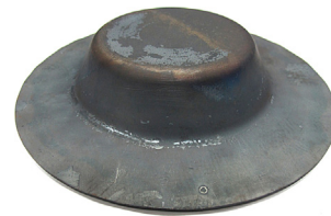
Fig. 6. Hot-stamped cup with water for t = 3 s.
