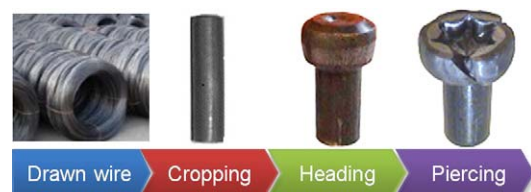
Fig. 2. Forging sequence for a C35 Torx-type socket screw.
