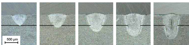
Fig. 2. Weld profiles at increasing ED: (a) \text{ED} = 20 \text{ J}/\text{mm}^2 , (b) \text{ED} = 25 \text{ J}/\text{mm}^2 , (c) \text{ED} = 31 \text{ J}/\text{mm}^2 , (d) \text{ED} = 36 \text{ J}/\text{mm}^2 , (e) \text{ED} = 49 \text{ J}/\text{mm}^2 .
