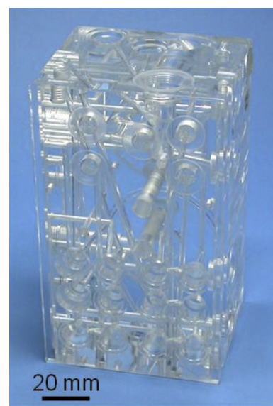
Fig. 1. Acryl glass model of a complex workpiece with intersection boreholes, Co. HELLER.
