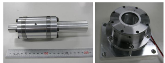
Fig. 4. The driving and the coil units.
