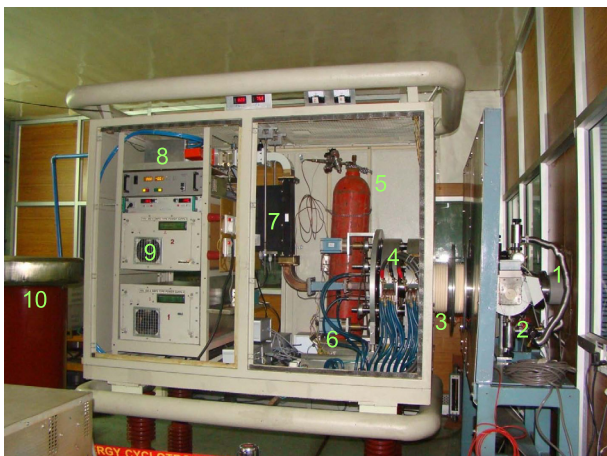
Fig. 1. 2.45 GHz microwave ion source on the 100 kV high voltage deck. (1) DCCT; (2) turbo pumps; (3) ceramic insulators to isolate HV deck; (4) solenoid coils; (5) \text{H}_2 gas cylinder; (6) motor assembly to move solenoids; (7) auto tuner; (8) magnetron and its power supply; (9) solenoid power supplies; (10) isolation transformer.
