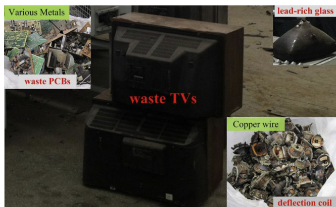
Fig. 1. Waste TVs and the contained components.
