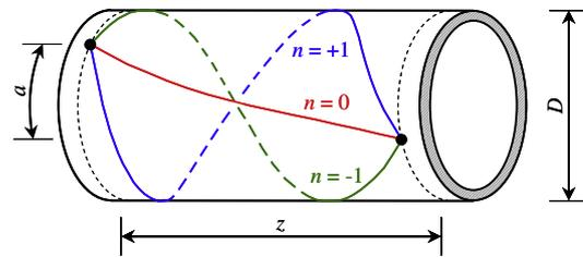
Fig. 1. A schematic view of the three lowest-order helical paths in a cylindrical pipe.
