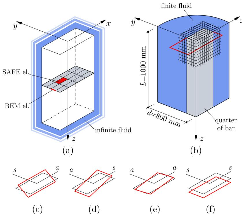
**Fig. 1.** SAFE–2.5D BEM model (a), Abaqus model (b) and boundary conditions for: slow flexural modes (c), fast flexural modes (d), torsional modes (e) and longitudinal modes (f). Axes of symmetry are indicated with  $s$ , while axes of antisymmetry are denoted with  $a$ .
