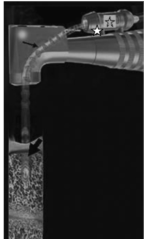
Fig. 2. A schematic representation of ultrasound measurement device. The ultrasonic waves from the ultrasonic transducer (☆) are propagated through a jet of water (thin arrow) into the drilled tract in bone (thick arrow) and reflected back via the same jet into the signal processor device (☆).
